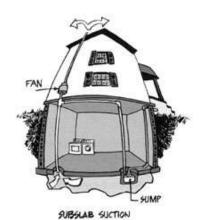
usually reduced by one of four types of soil suction: subslab suction, drain tile suction, sump hole suction, or block wall suction. Active subslab suction (also called subslab depressurization) is the most common and usually the most reliable radon reduction method. One or more suction pipes are inserted through the floor slab into the crushed rock or soil underneath. They also may be inserted below the concrete slab from outside the house. The number and location of
